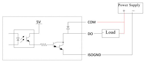
Figure 4.1 Schematic diagram of digital output circuit
