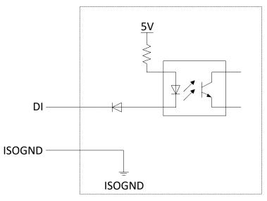
Figure 3.1 Schematic diagram of digital input circuit
