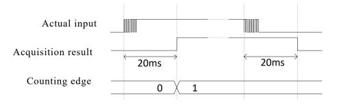
Figure 3.4 The schematic diagram of rising edge counting principle
