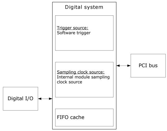
Figure 1.1 PCI-1316 data acquisition device functions
