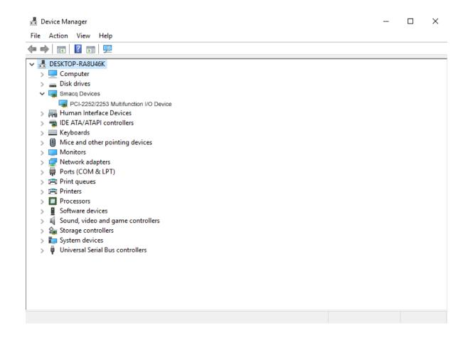
Figure 2.7 Device Manager after successful driver installation
