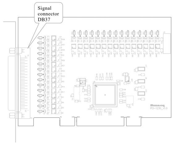
Figure 2.1 Schematic diagram of PCI-1232 digital output control card
