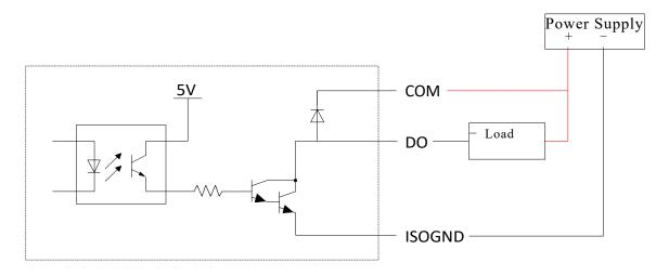
Figure 3.1 Schematic diagram of digital output circuit
