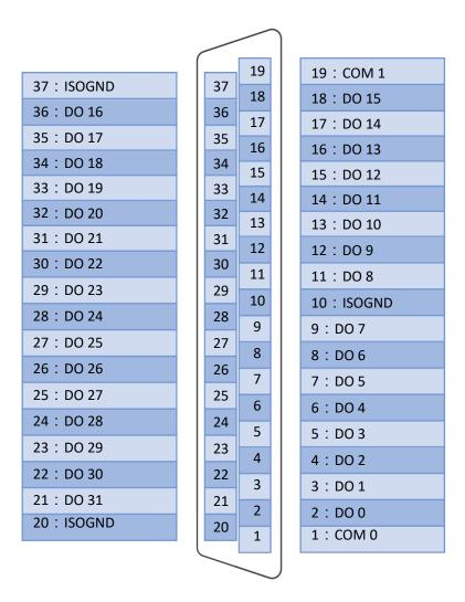
Figure 2.1 Signal connector distribution diagram
