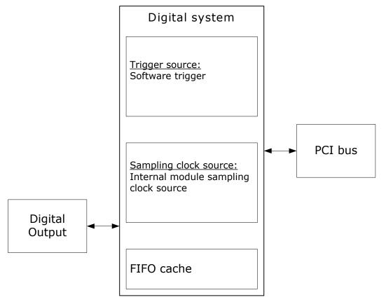
Figure 1.1 PCI-1232 data acquisition device functions
