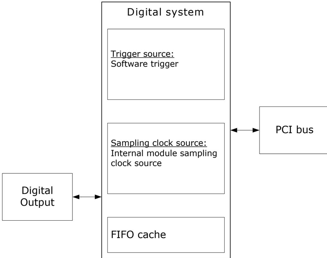
Figure 1.1 PCI-1232 data acquisition device functions
