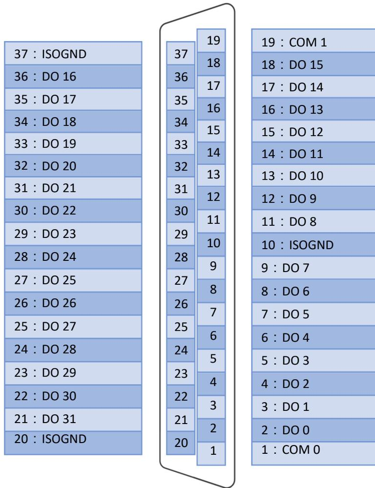
Figure 2.1 Signal connector distribution diagram
