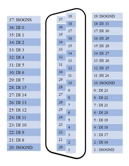
Figure 2.2 Signal connector distribution diagram
