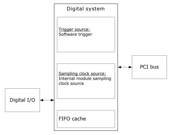
Figure 1.1 PCI-1132 data acquisition device functions
