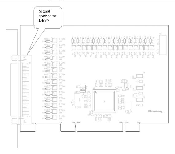
Figure 2.1 Schematic diagram of PCI-1132 digital input acquisition device
