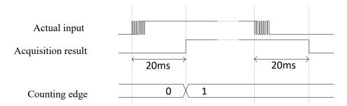
Figure 3.4 The schematic diagram of rising edge counting principle
