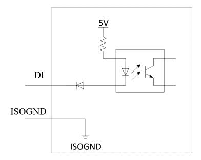
Figure 3.1, digital input circuit Figure
