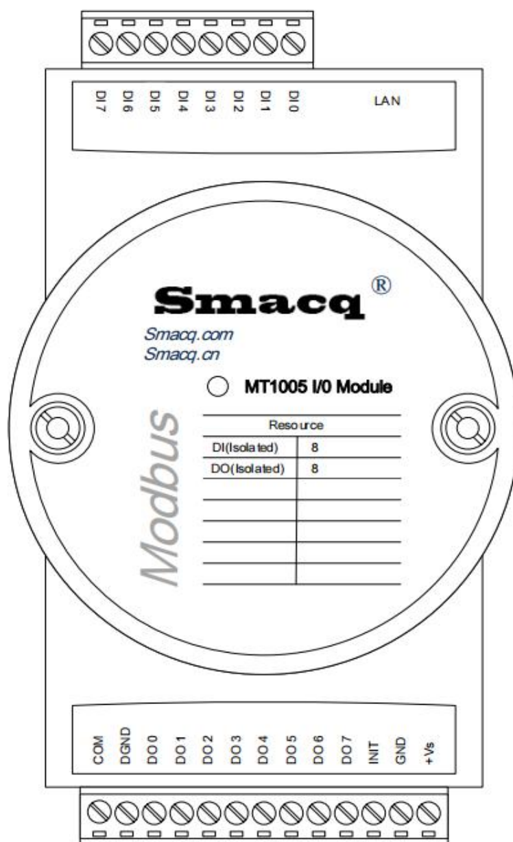
MT1005 Wiring Definition
